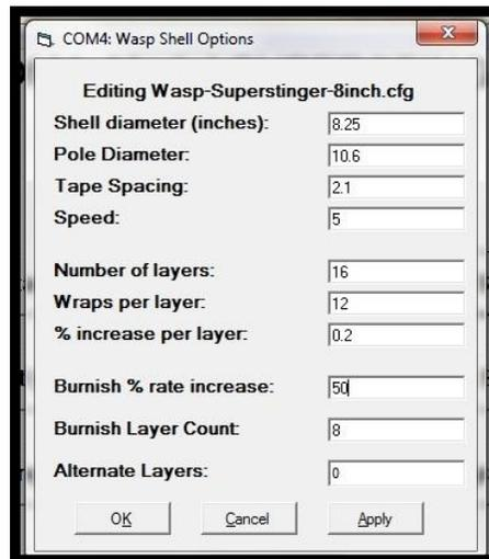
Once this program was set, I clicked “Apply” and then “OK” which brought up the main operations screen. I then clicked “Save this Shell” and named it “Wasp-7.5inch.cfg” to denote the casing diameter which it is designed for.
