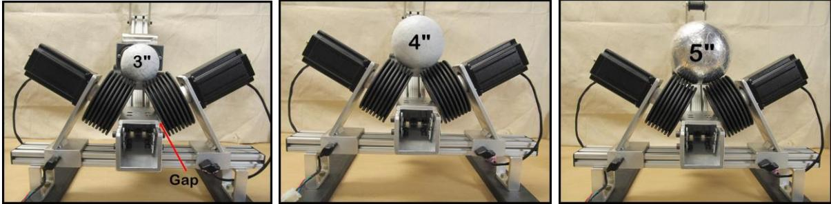
For 6" shells, increase those gaps to  $\frac{3}{8}$ ". You can see how that causes the shell to ride right in the middle of the drive rollers.
