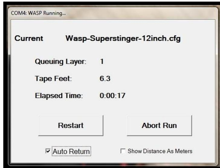
Clicking “Restart” will resume the taping program where it left off. Pausing is convenient when the roll of tape needs to be changed.
