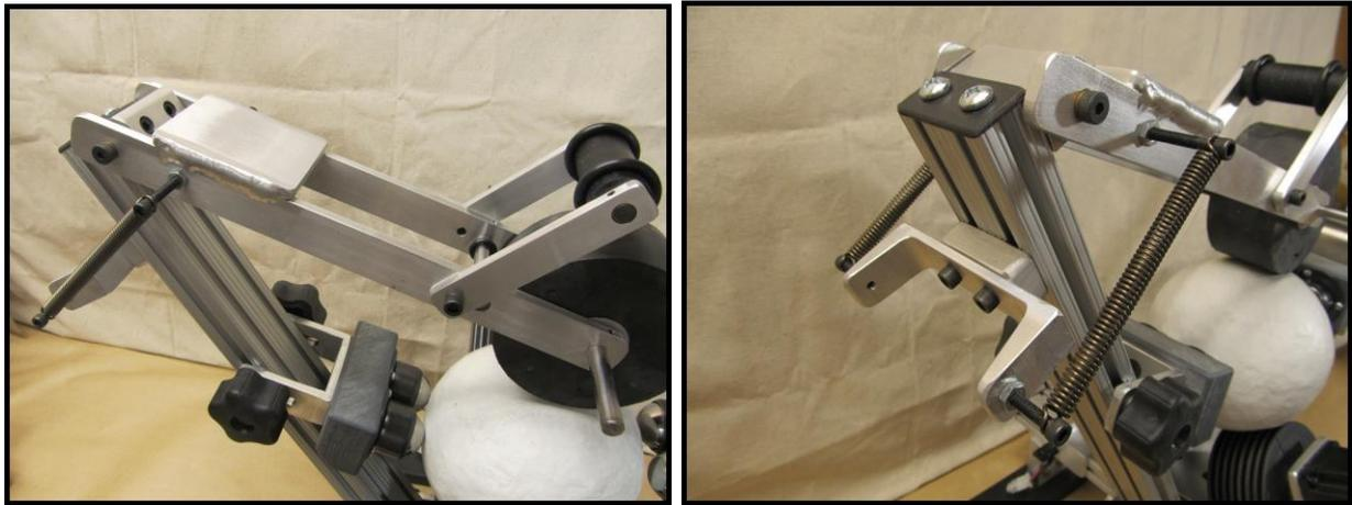
During taping, the tape-application wheel should ride centered slightly to the right of the shell’s centerline:
