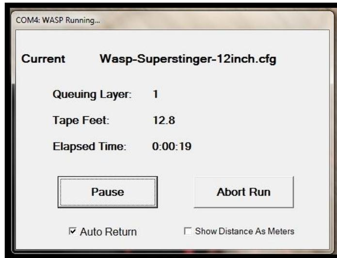
It shows what program is running, and the “Queuing Layer” counter will begin to count up, showing how many layers have been applied to the shell. “Tape Feet” and “Elapsed Time” will also count up.
