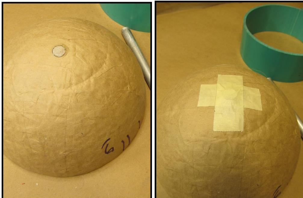
The inside end of the passfire tube is then sealed off with a piece of tissue paper, hot-glued in place, to prevent stars or burst charge from falling into the tube during shell assembly.
