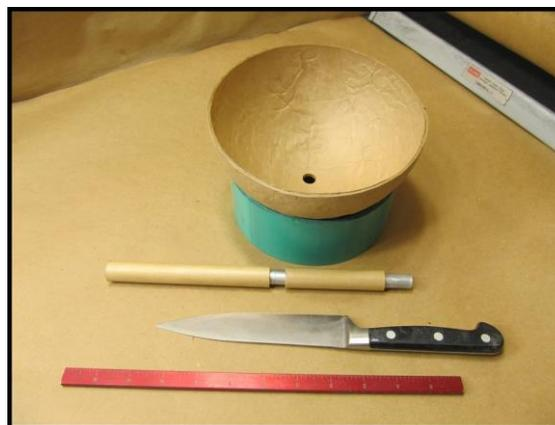
After a 1/2" dowel is inserted into the casing's hole, the passfire tube is slid down over it, and hot-glued to the inside of the hemisphere.
