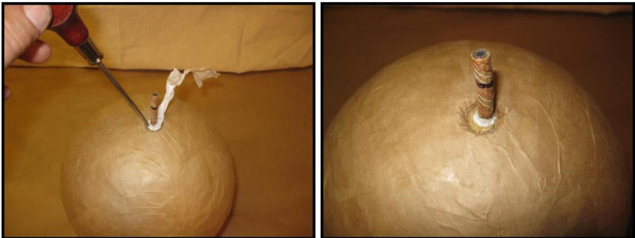
Now, the purpose of the two methods described below is to seal that hole in the shell's casing around the fuse. Making a solid, strong seal which will
