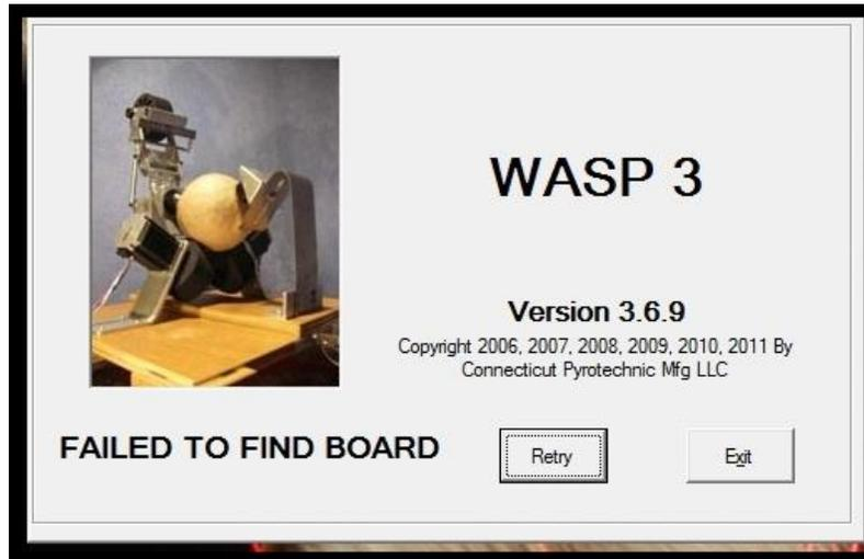
If that occurs, check all the cables, especially the USB cable from the controller to the computer, and the 110 volt power line to the power-supply, and click "Retry". If that doesn't solve the problem, click "Exit", check all the cables again, and open the program again, hopefully arriving at the "COM4: Model WASP3" window.
